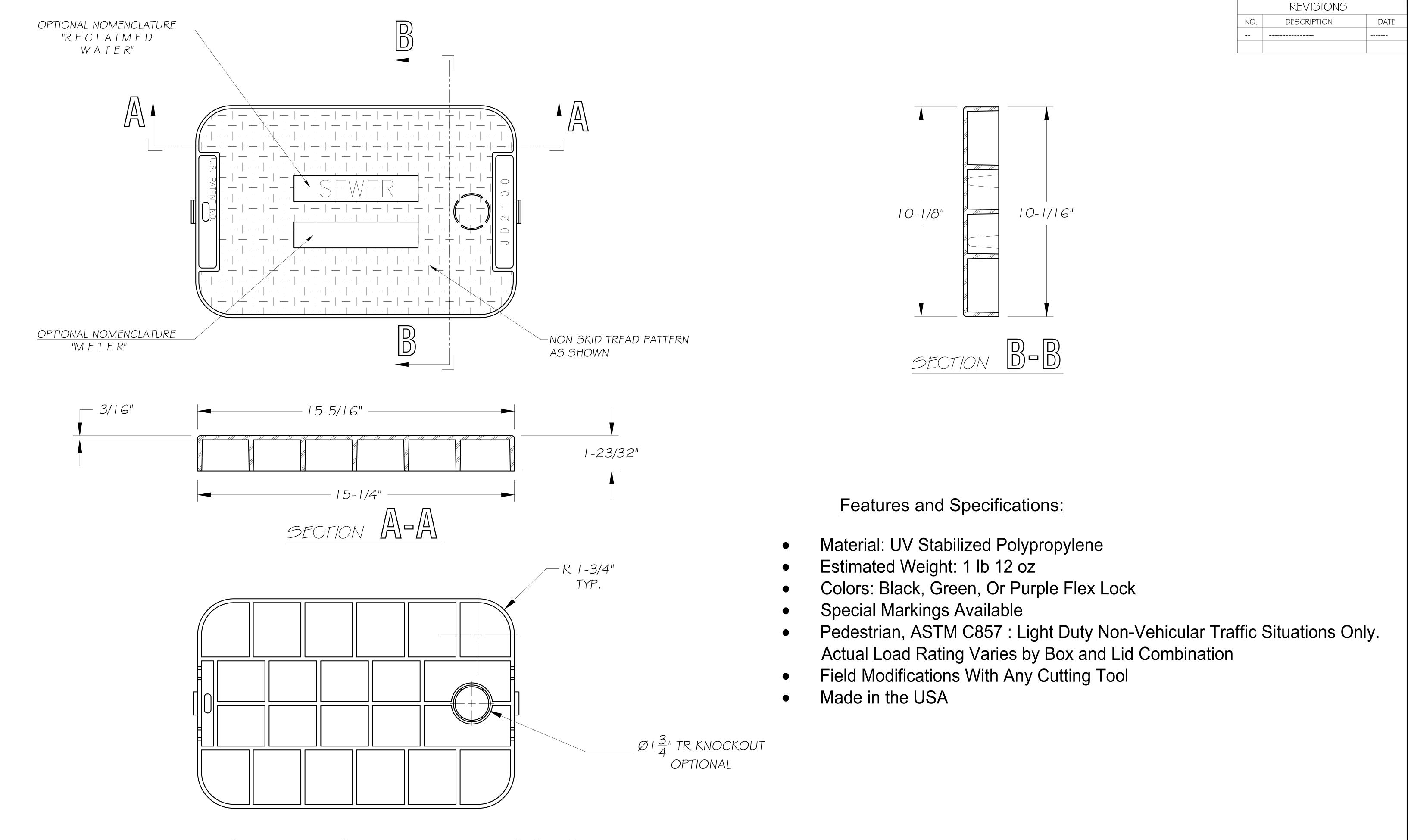
JD2102SBL ~ 1-3/4" DIA. TR KNOCKOUT RECESSED FLUSH COVER
